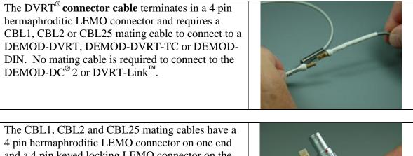
The CBL1, CBL2 and CBL25 mating cables have a 4 pin hermaphroditic LEMO connector on one end and a 4 pin keyed locking LEMO connector on the other with a red dot for alignment.
