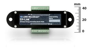
EH-Link® - versatile multi-sensor node that runs on ambient energy sources such as vibration, light, and thermoelectric
