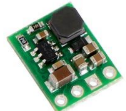
Figure 2: Step-down Voltage Regulator
